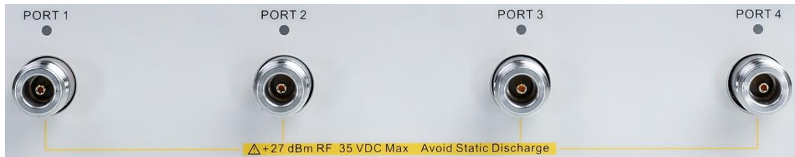
Figure 1-6 Front panel RF connectors (4-port VNA)
