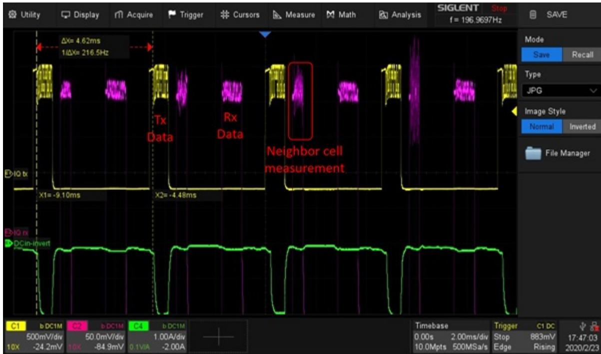
Figure 7: Call Tx and Rx bursts
