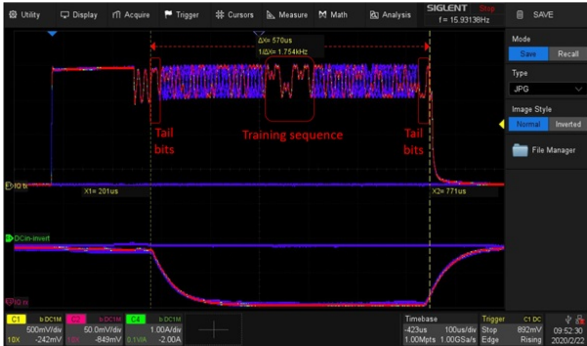
Figure 8: Histogram of Tx signal with 1-sec persistence
