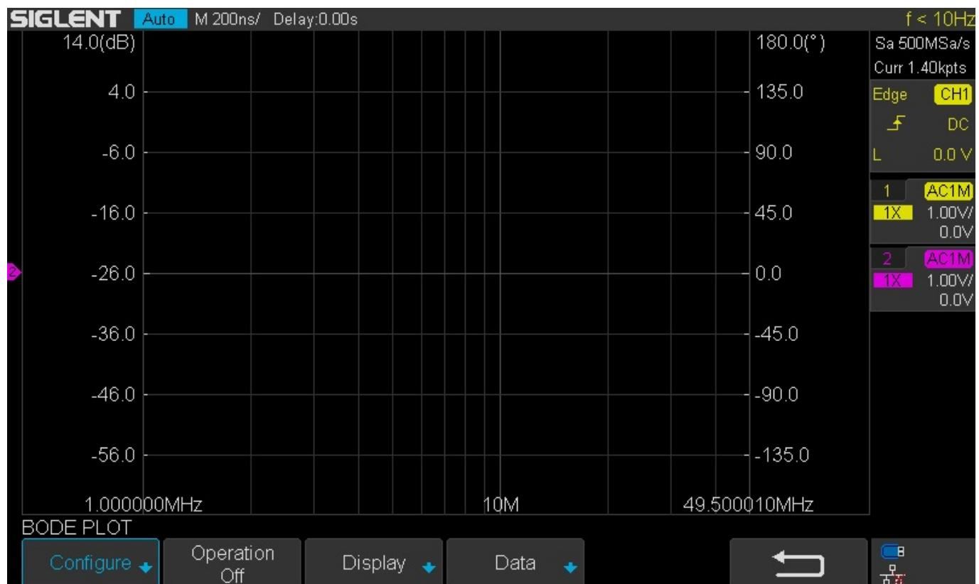
2. Press Configure to open up the generator Configure (AWG) controls and sweep parameters:
