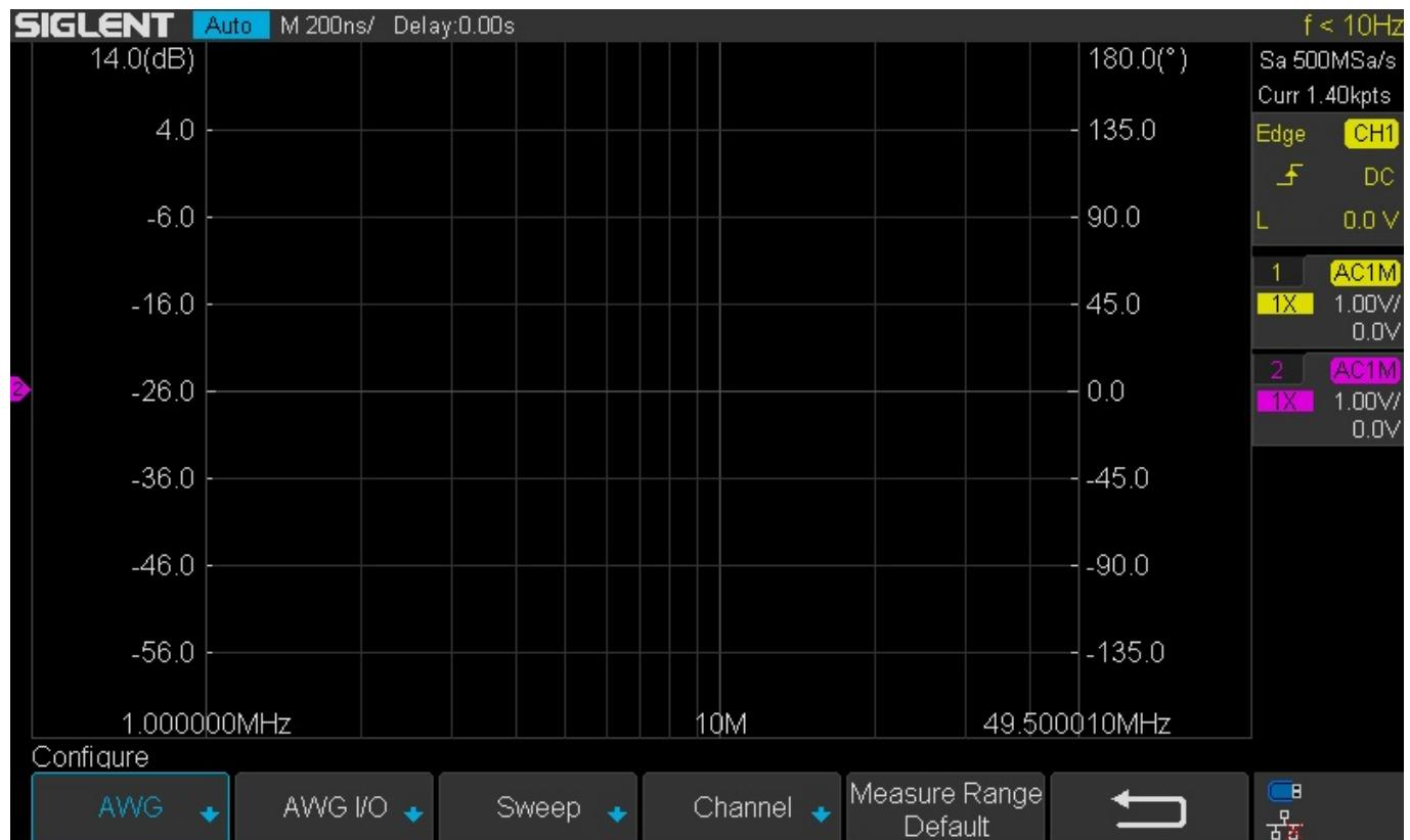
3. Press AWG to set the signal amplitude and set expected device load impedance. Press the back arrow to return to the Configure screen.
