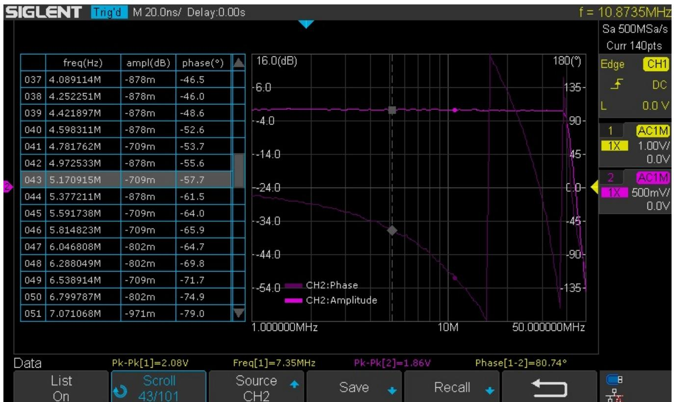
From here, you can use the scroll and cursors to find individual data points, quick print display images to USB, and save CSV data to USB using the Save function.
