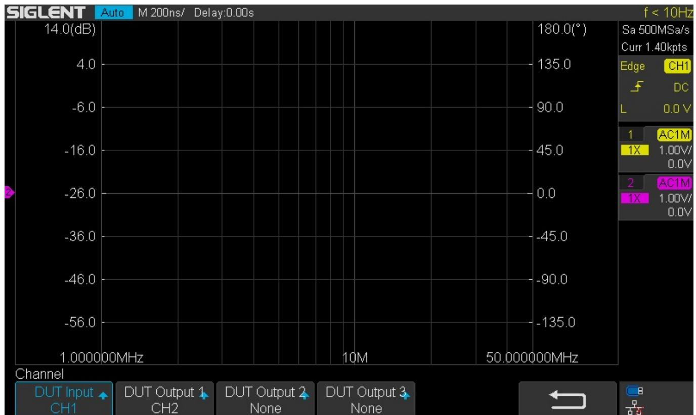
Here, you can see we have DUT input (the direct signal from the generator) connected to Oscilloscope channel 1. The scope CH2 is connected to the DUT output (the through connection).
