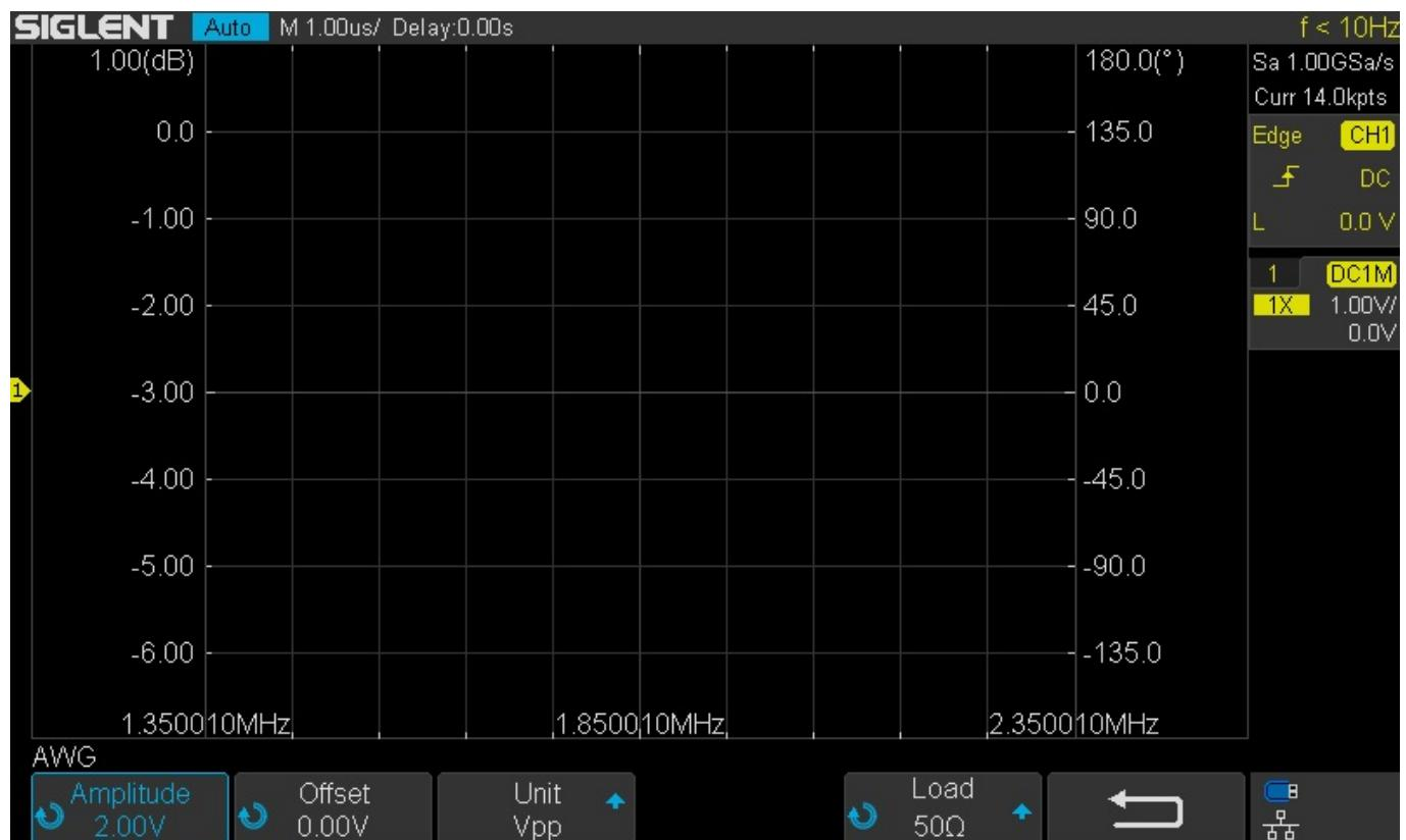
4. Press Sweep to open the Sweep menu. Here, you can set the mode, sweep start/stop frequencies and resolution:
