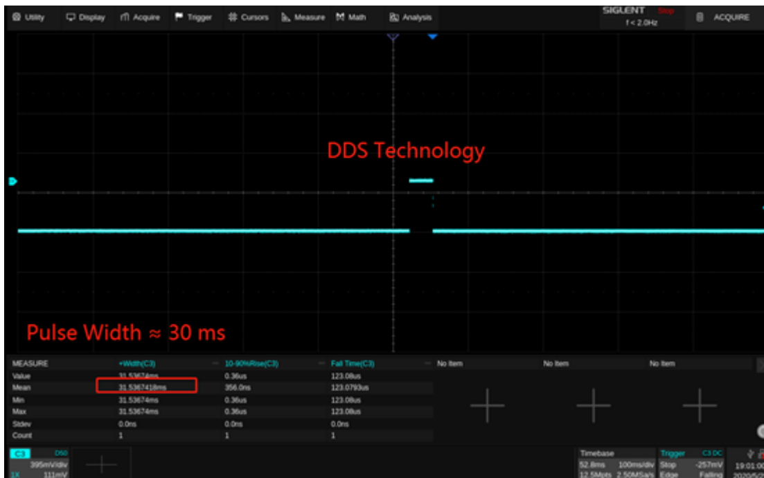
Figure 6: 1 Hz pulse signal generated by DDS
