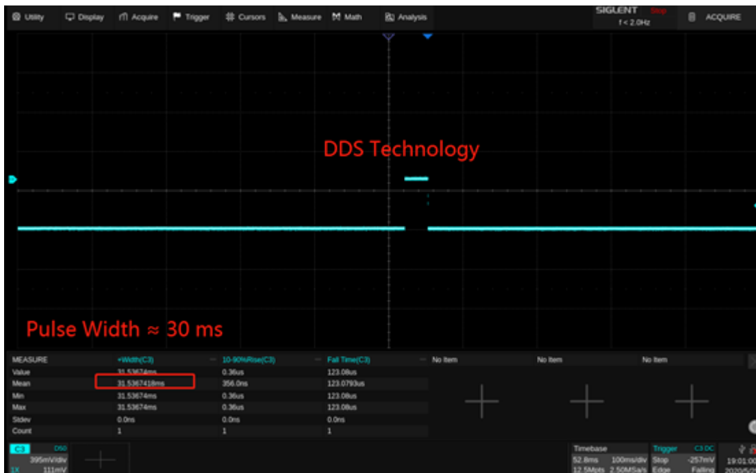
Figure 6: 1 Hz pulse signal generated by DDS
