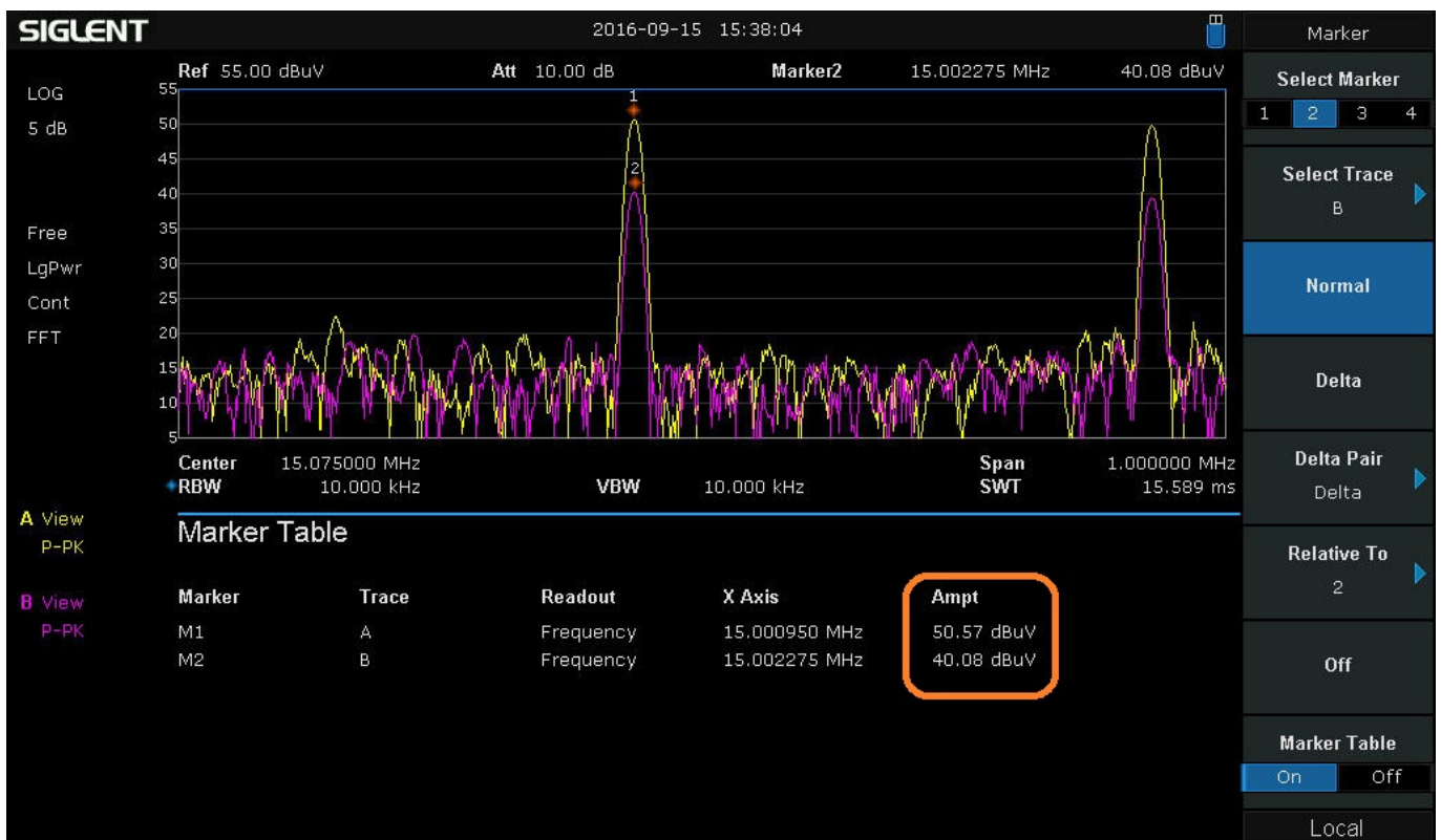
Figure 5: Comparison of two scans using the marker table function of the SIGLENT SSA3000X spectrum analyzer. The Yellow trace was collected without attenuation while the Pink trace was collected after adding a 10 dB external attenuator.
