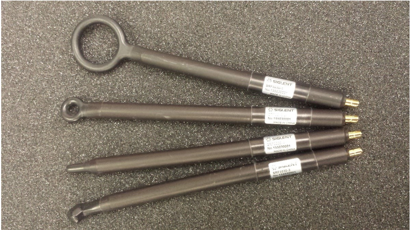
Figure 3: Siglent SRF5030 Near-Field Probe kit includes 2 loop and 2 point magnetic (H) field probes, cable, and adapter. Only the probes are shown.
