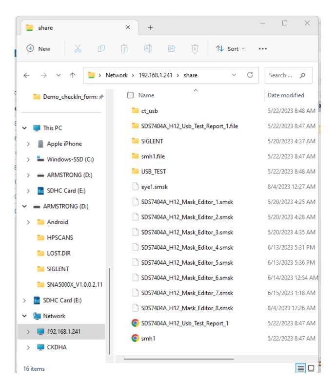
On the SDS2000X HD, SDS6000A, or SDS7000A you may also mount a drive from your PC. This is called SMB File Share CLIENT mode.
