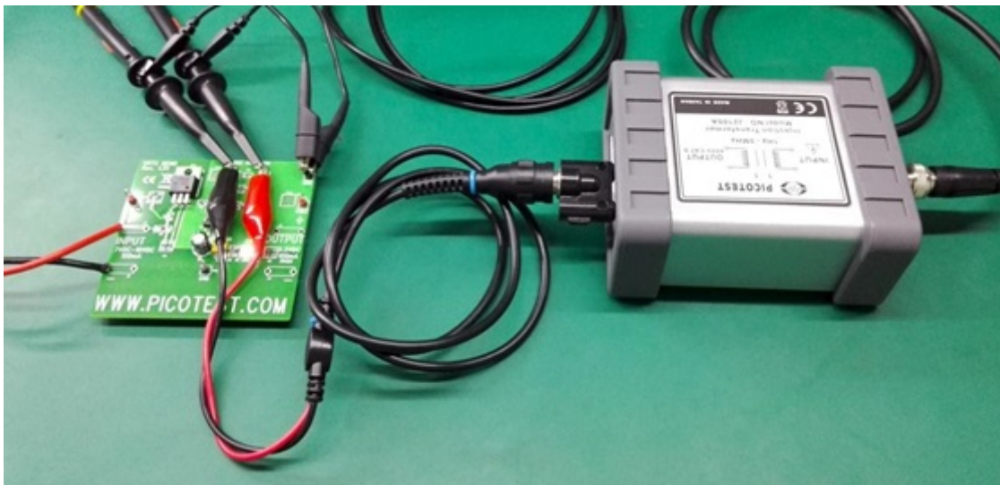
Figure 9: Probe and Transformer connections to the DUT
