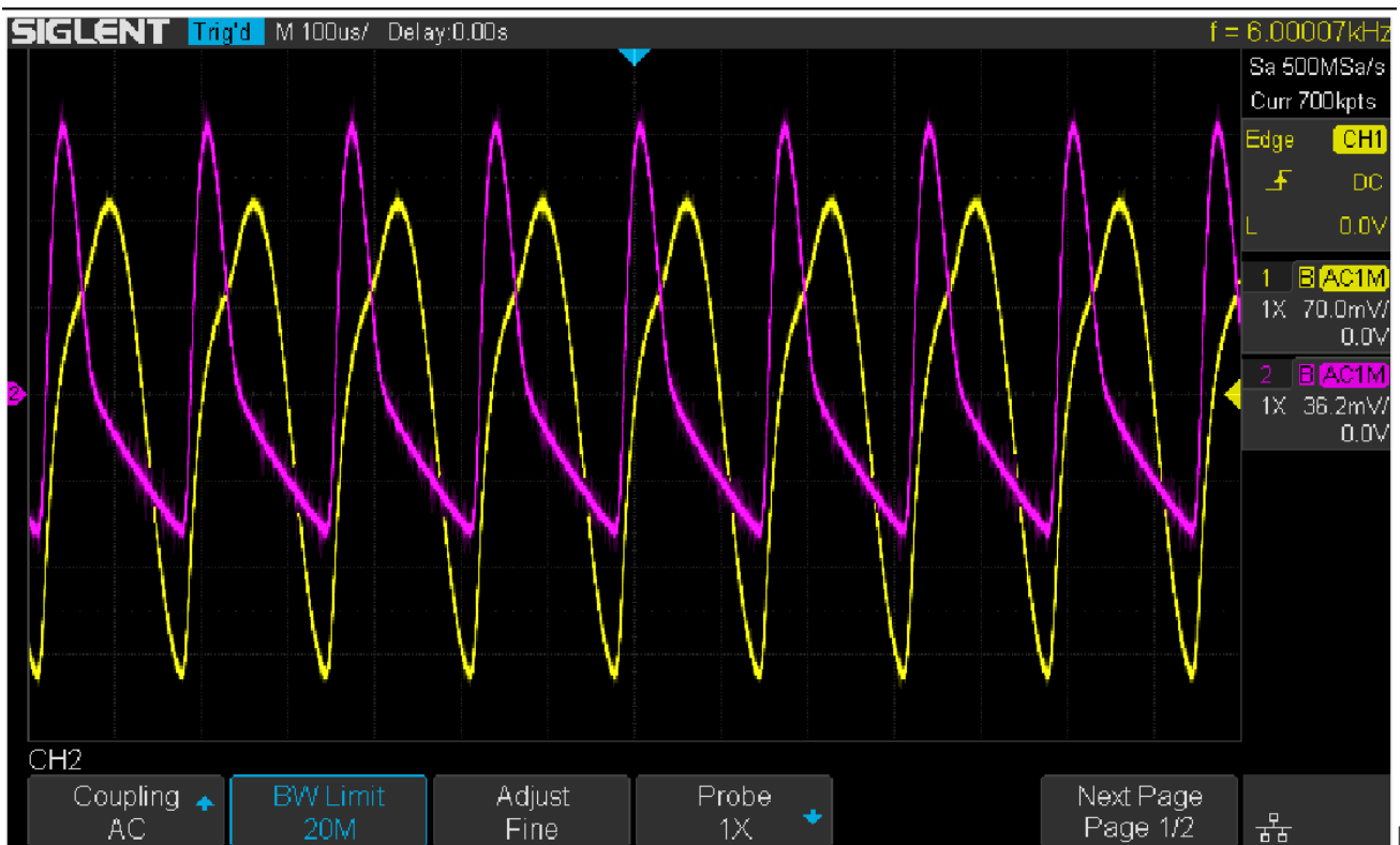
Figure 15: Distortion in the time domain
