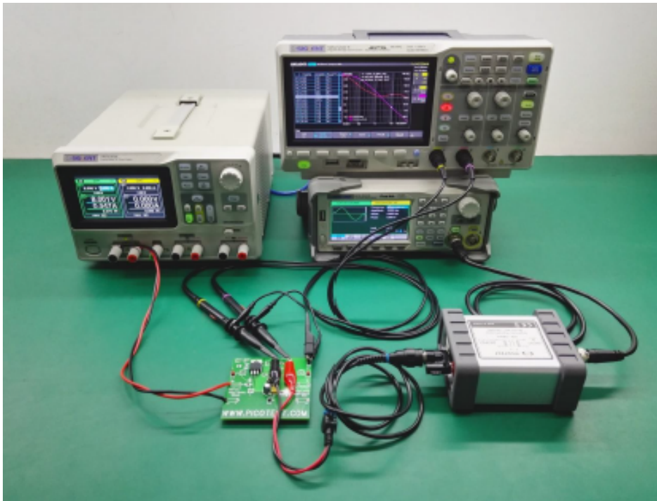
Figure 1: Bode II setup
