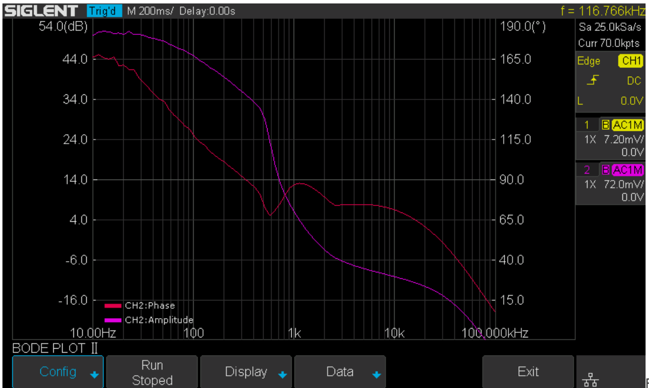
Figure 14: Increased stimulus signal amplitude and distortion
