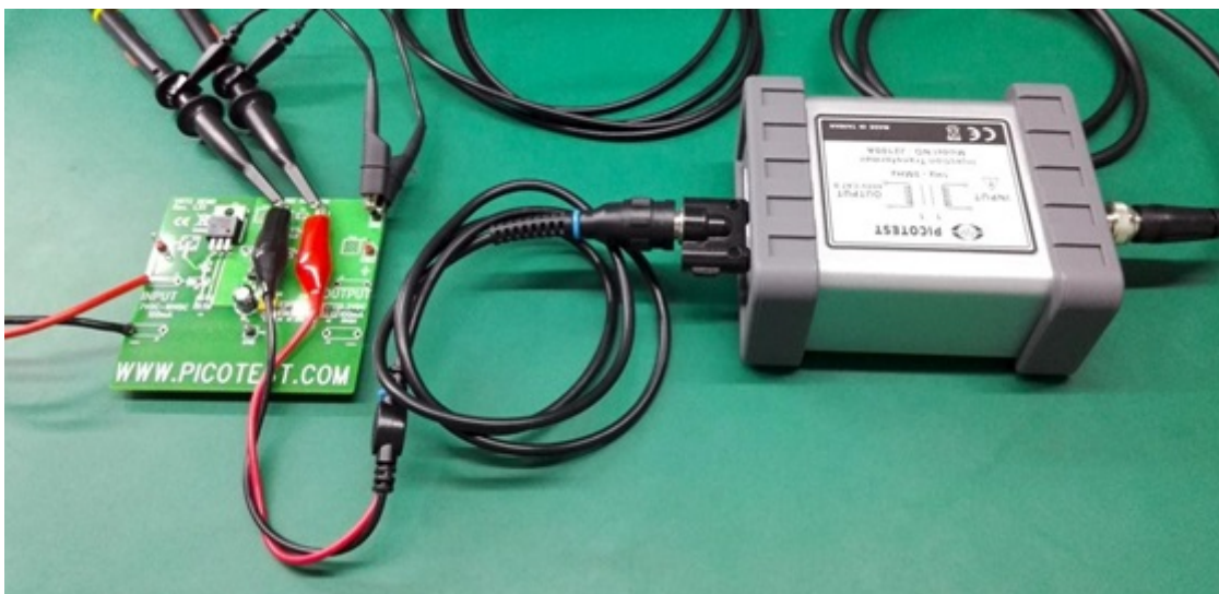
Figure 9: Probe and Transformer connections to the DUT
