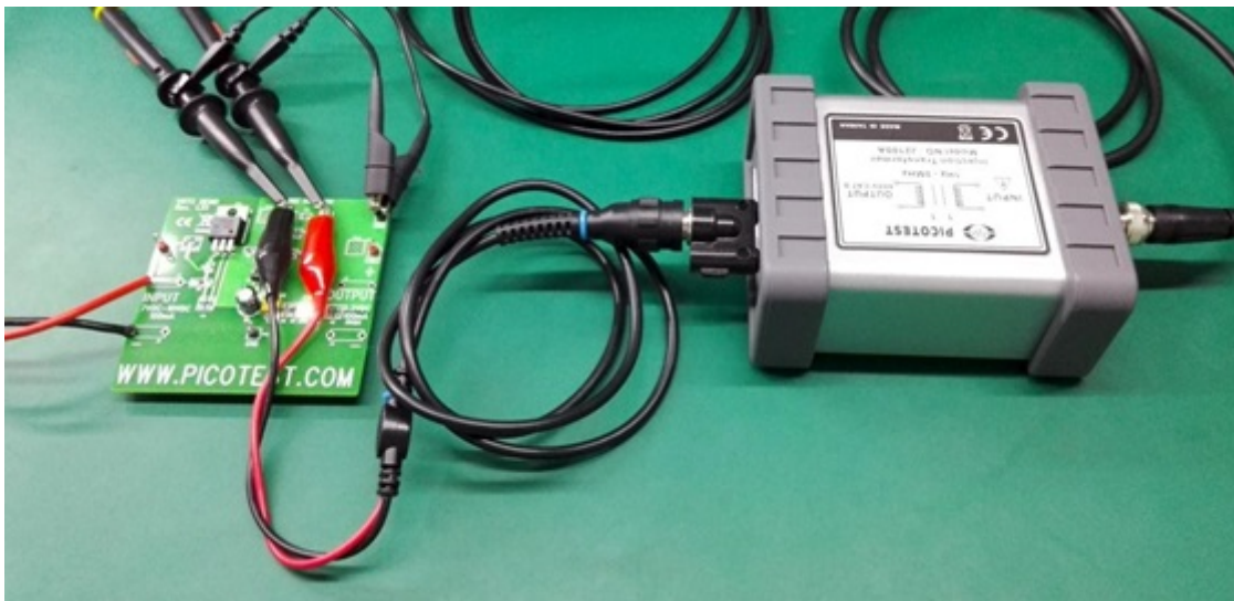
Figure 9: Probe and Transformer connections to the DUT
