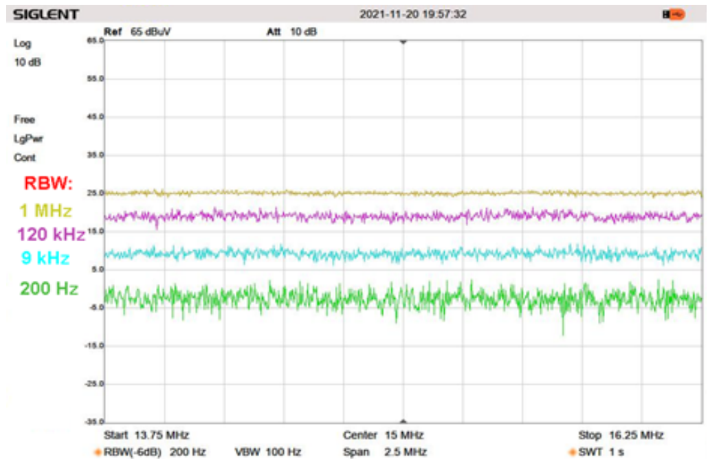
Figure 3: Spectrum analyzer DANL level versus resolution bandwidth.
