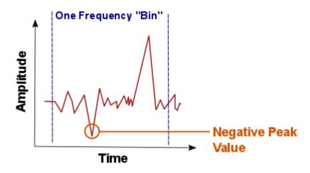
Negative peak detectors are rarely used, but can be helpful when comparing positive and negative peak values when looking for CW and Pulsed signals. CW signals will have less difference between positive and negative peak values for a given frequency bin. A pulsed signal could have a significant difference
