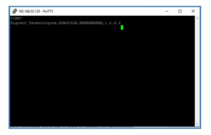
This is the standard command string that is used to request the identification string from the instrument. As shown below, the instrument responds with the manufacture, product ID, Serial Number, and firmware revision.
