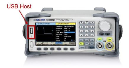
2. Press the Utility key on the front panel, and then softkey "System ->Page 1/2 -> Firmware Update", to enter the interface of the file browser.
