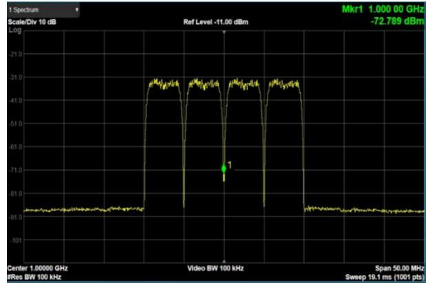
ARB mode to add real time AWGN to digital IQ signals for receiver performance tests
