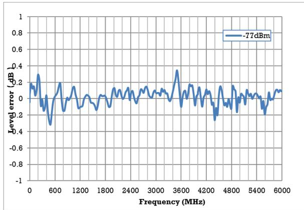
Measured level error versus frequency,
