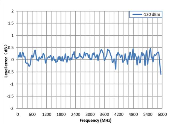
Measured level error versus frequency,
