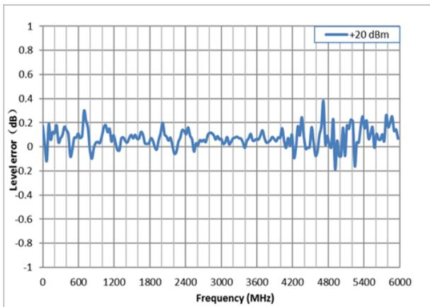
Measured level error versus frequency,
