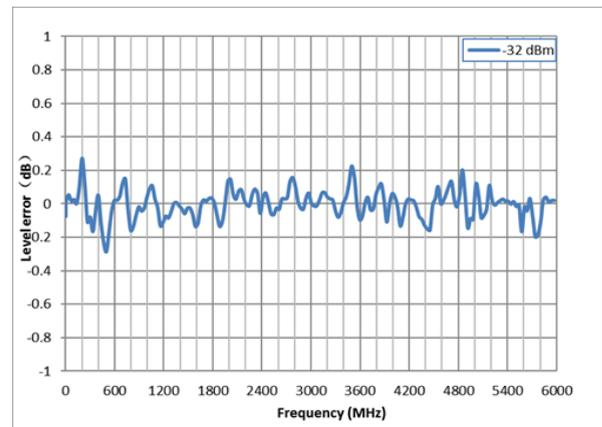
Measured level error versus frequency,
