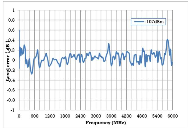
Measured level error versus frequency,
