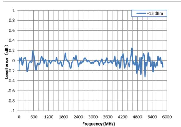
Measured level error versus frequency,
