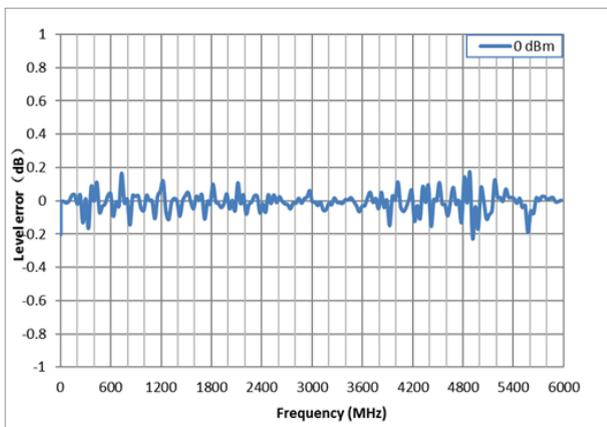
Measured level error versus frequency,
