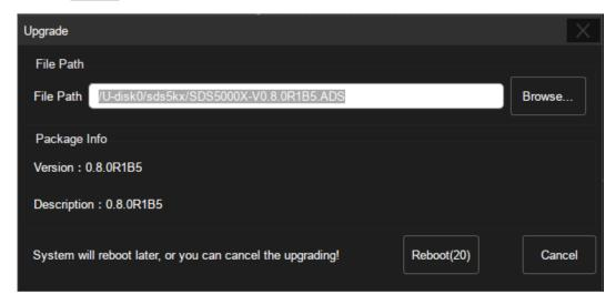
6. After the instrument reboots, check the version number through the Utility->System Setting->System Status to confirm if the upgrade is successful.
