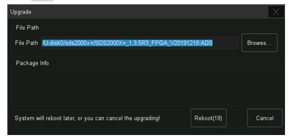
After the instrument reboots, check the version number through the Utility->System Setting->System Status to confirm if the upgrade is successful.
