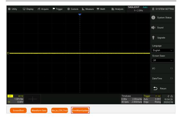
Select the correct update file (\*.ads) stored on the computer. The instrument will automatically download the update file and perform the upgrade once the file is specified.
