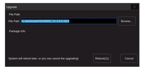
6. After the instrument reboots, check the version number through the Utility->System Info to confirm if the upgrade is successful.
