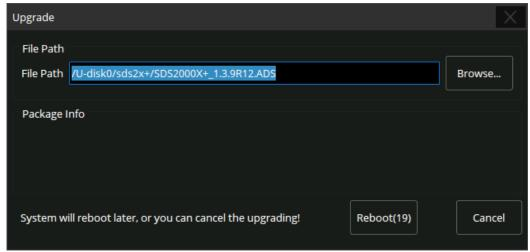
After the instrument reboots, check the version number through the Utility-> System Info to confirm if the upgrade is successful.
