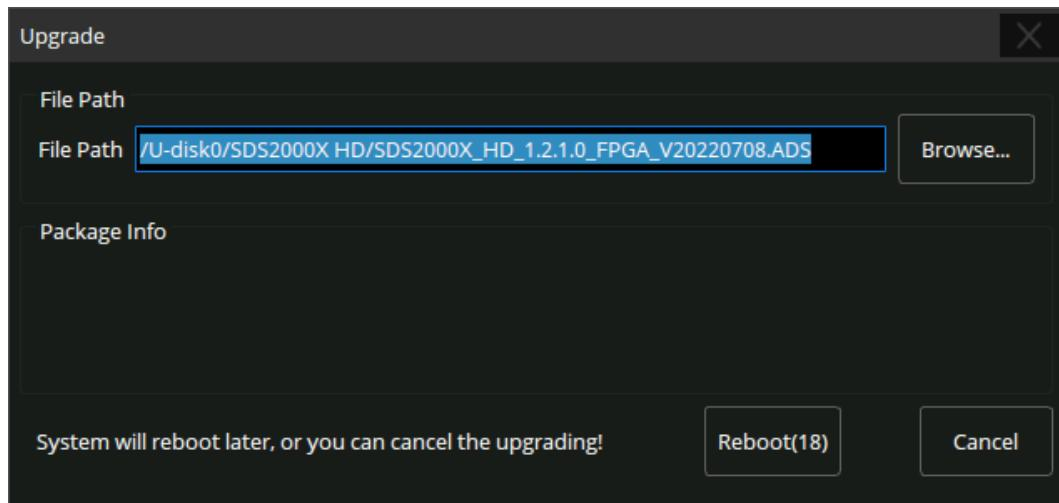
6. After the instrument reboots, check the version number through the steps **Utility** -> **Menu** -> **System Info** to confirm if the upgrade is successful.
