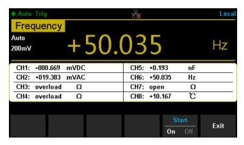
The upper part of the interface displays the function, range, and result of the current channel. The table below records the measurement result of each channel.
