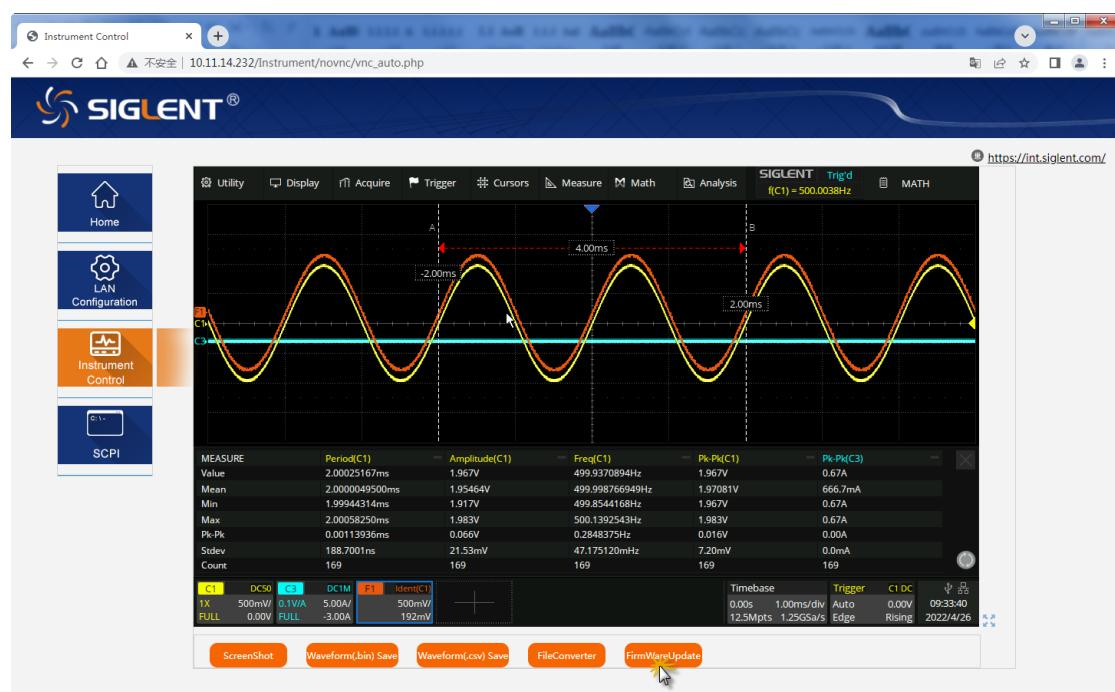
2. Select the correct update file (\*.ads) stored on the computer. The instrument will automatically download the update file and perform the upgrade once the file is specified.
