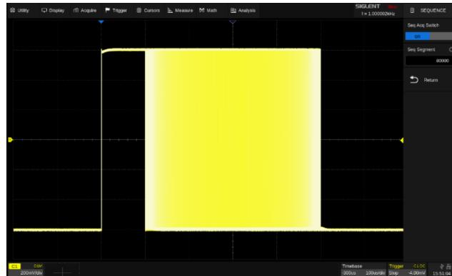
Segmented memory collection will store the waveform into multiple memory segments (up to 80,000) and each segment will store a triggered waveform as well as the dead time information. The interval between segments can be as small as 1.3μs. All of the segments can be played back using the History function.
