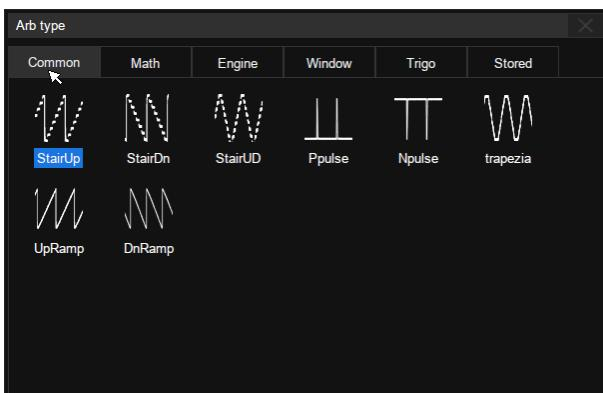
The built-in Function / Arbitrary waveform generator can output waveform with up to 25 MHz frequency and  $\pm 3V$  amplitude. Six basic waveforms plus multiple types of arbitrary waveforms are built-in.
