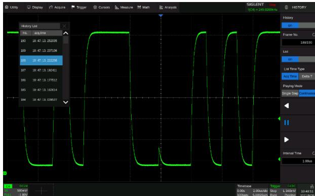
The history function can record up to 80,000 frames of waveforms. The recording is executed automatically so that the customer can playback the history waveforms at any time to observe unusual events and quickly locate the area of interest using cursors or measurements. The failed frames of the Mask Test can be stored as history frames.
