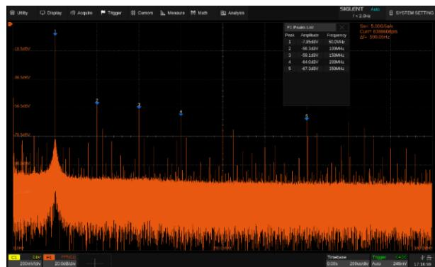
Hardware-accelerated FFT supports up to 8 Mpts operation. This provides high-frequency resolution with a fast refresh rate. The FFT function also supports a variety of window functions so that it can adapt to different spectrum measurement needs. Three modes (Normal, Average, and Max hold) can satisfy different requirements for observing the power spectrum. Auto peak detection and markers are supported.
