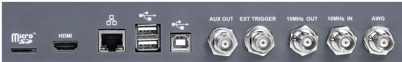
HDMI (1280 x 800) x1, USB Host 3.0 x2, USB Host 2.0 x2, USB Device 2.0 (USBTMC) x1, 1000M LAN (VXI-11 / Telnet / Socket)x1, micro SD card x1, Auxiliary output (Pass / Fail, Trigger Out) x1, 10 MHz In x1, 10 MHz Out x1
