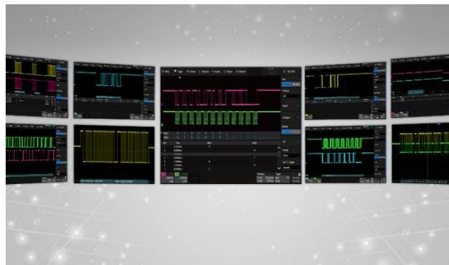
Display the decoded characters through the events list. Bus protocol information can be quickly and intuitively displayed in tabular form. I2C, SPI, UART, CAN, LIN, CAN FD, CAN XL, FlexRay, I2S, MIL-STD-1553B, SENT, ARINC429, SpaceWire, USB2.0 and Manchester are supported.
