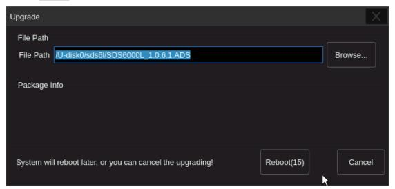
After the instrument reboots, check the version number through the *Utility* -> *Menu* -> System Info to confirm if the upgrade is successful.
