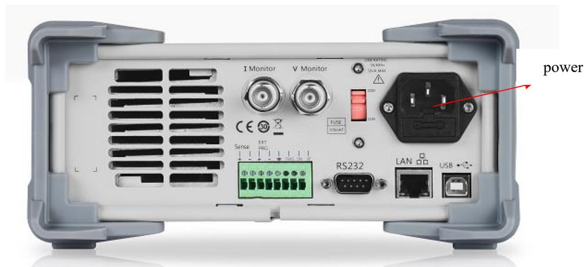
Figure 1-1 connect the power cord
