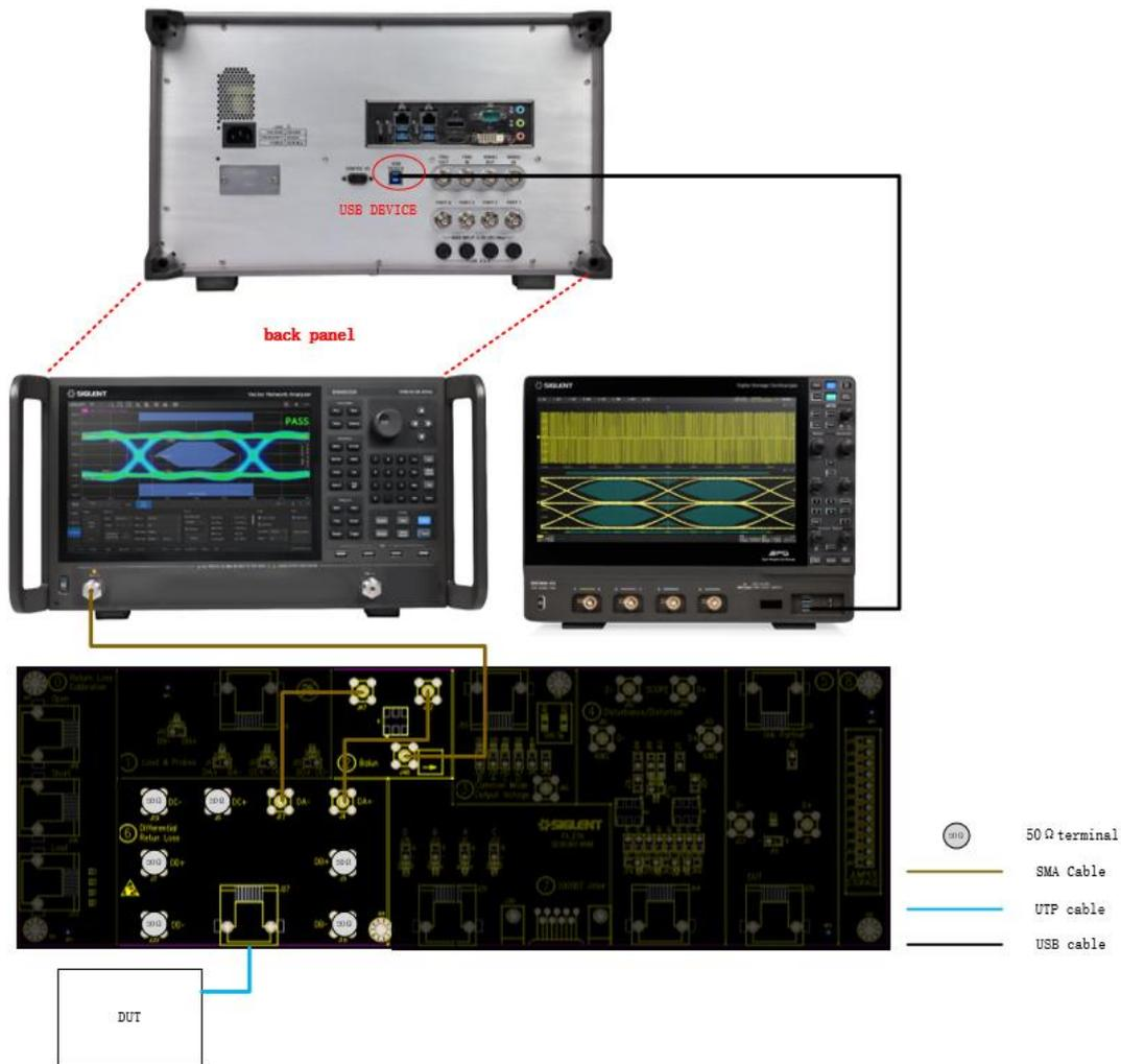
Figure 6-18 Transmitter Return Loss Test Environment
