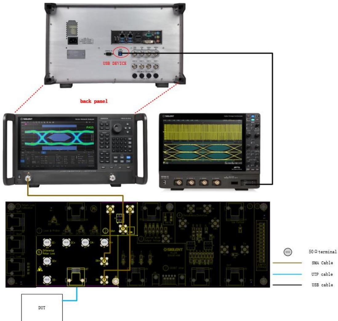
Figure 6-22 Receiver return loss test connection
