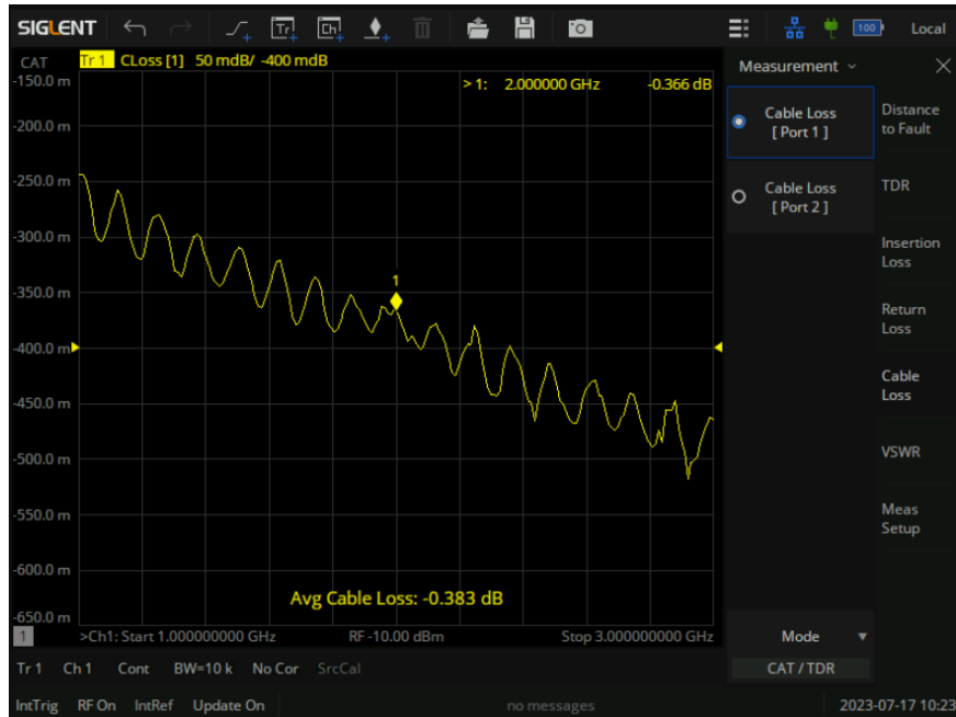
Figure 13-8 Cable loss measurement interface
