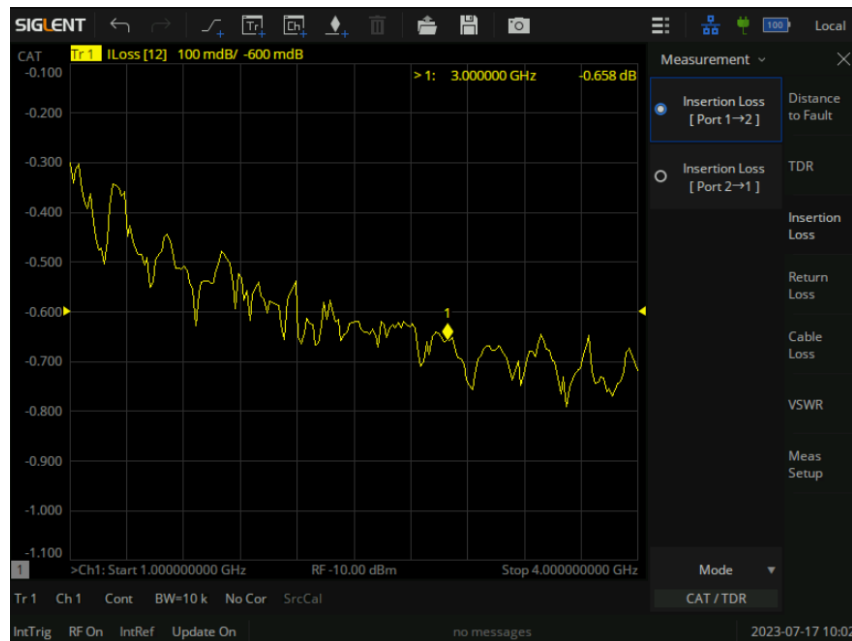
Figure 13-6 Insertion loss measurement interface
