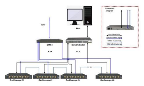
Very large systems are really defined by use of the SYN64 trigger box. This device makes it possible to trigger up to 64 oscilloscopes with low jitter. This requires a clean trigger event incoming for parallel capture. Using this box, the trigger can be scaled up
