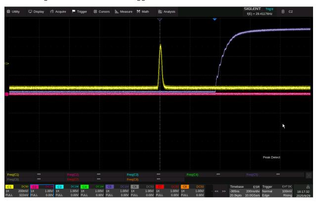
Persistence is set to infinite here, so you can see the trigger jitter on the yellow pulse is very small, on the order of ~10 nanoseconds. We also see that the trigger signal in purple arrives about 370 nanoseconds after the pulse in this setup. This is heavily dependent on the cable lengths, probing, and wiring scheme but in this case, most of that is within the master instrument.
