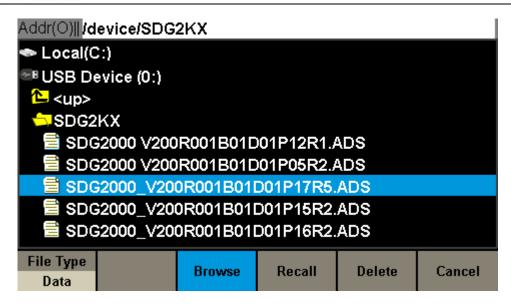
4. Press "Recall" to start the update. A progress bar is displayed during the update. After the update is completed, the generator will restart automatically.
