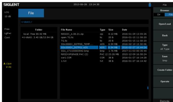
4. Press “Open/Load” to start the update. A progress bar is displayed during the update. When updating complete, the spectrum analyzer will restart automatically.
