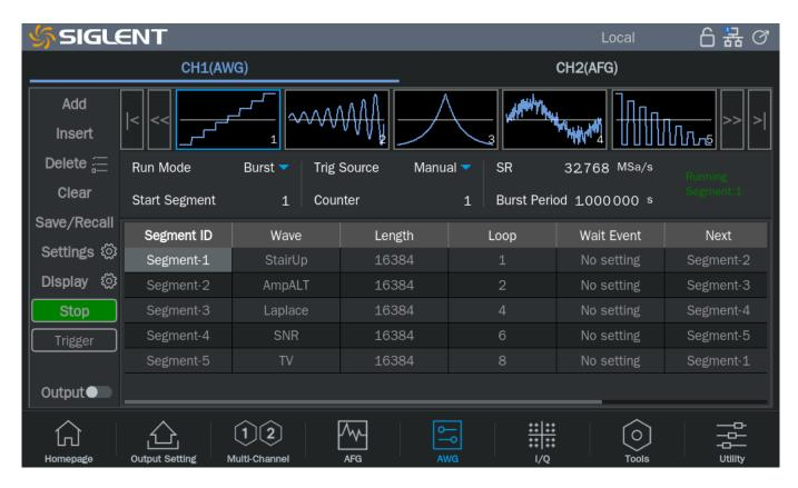
It supports PRBS signal output up to 120 Mbps, baseband and IF IQ signal generation with symbol rates from 250 to 50 MSymb/s, and a wide range of modulation types including AM, DSB-SC, FM, PM, FSK, ASK, PSK, and PWM. With built-in Sweep and Burst modes, the SDG3000X delivers comprehensive support across a variety of test environments—from education and R&D to industrial power device testing.
