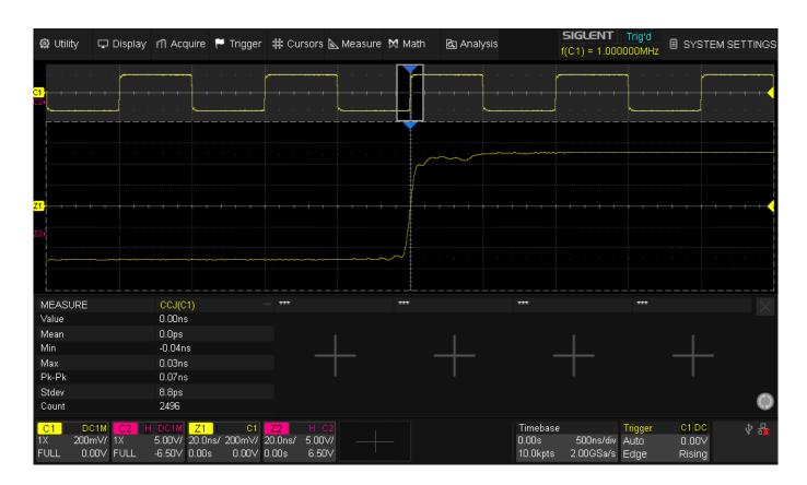
TrueArb enables point-by-point waveform generation across a sampling range of 10 mSa/s to 600 MSa/s, maintaining waveform integrity while delivering ultra-low jitter (as low as 150 ps) and total harmonic distortion (THD) below 0.075%, ensuring superior signal fidelity.
