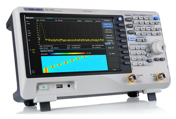
SIGLENT Technologies presents the SVA1032X as a novelty from the product group of spectrum & vector analyzer. Compared to SVA1015X, not only frequency range is extended, but also performance and RF specs. The spectrum analyzer frequency range is 9 kHz – 3.2GHz, vector network analyzer frequency range is 100 kHz – 3.2 GHz. Furthermore, the optional vector network analysis (VNA) function will be included in the SVA1015X model as also standard.
