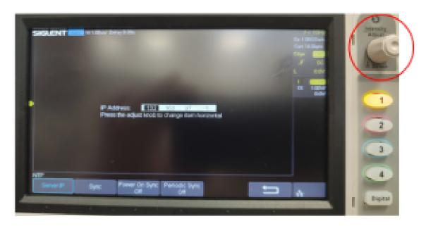
• After setting the IP Address, press *Sync* The status message shown below appears at the bottom of the screen.
