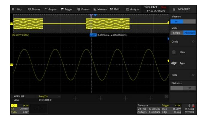
Here is an example of a more complex pulse train. Here, the pulse train contains 50 periods, and the pulse train repeats every second. Basically 50-period bursts of RF per second. In this example, we use an external signal to trigger the burst of pulses.
