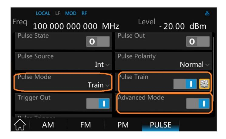
The Advanced Pulse Train feature lets you set the On, Off, Count, Frequency, and level of each pulse for even more flexible pulse source options:
