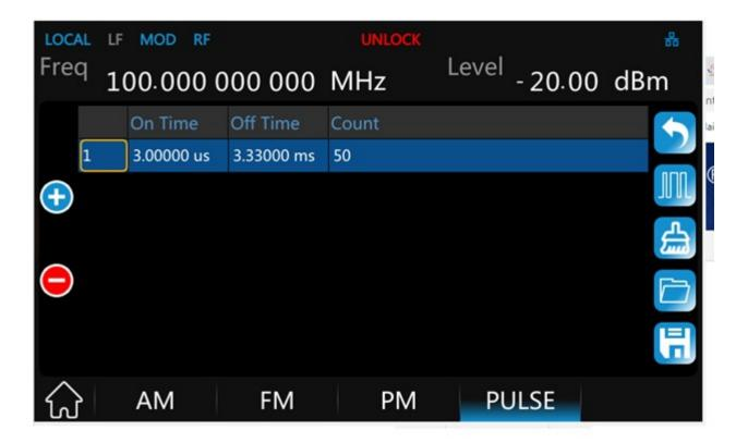
And the Ext Trigger (0-5V at the rear panel of the SSG) will trigger the pulse train:
