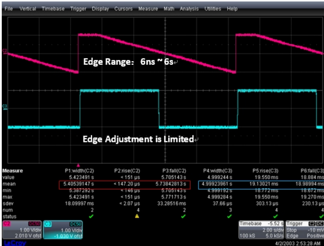
P3 Comparison of edge adjustment of low frequency 0.1Hz pulse signal
