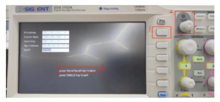
Firstly, press the button(1) and rotate the knob(2), which will select using DHCP or not. And press Save/Recall button to save the IP settings. (I am using DHCP and the IP address is 10.11.21.4)
