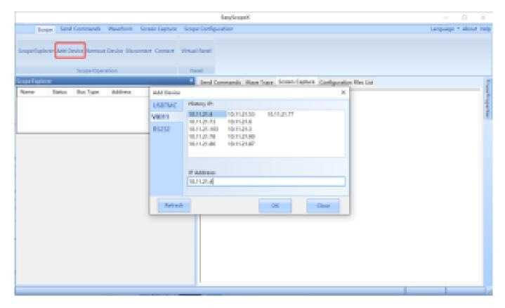
Secondly, open the EasyScopeX, select Add Device and type the IP address in VXI11, click OK.
