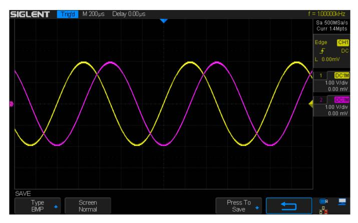
Step 1: Send "MEAD PHA,C1-C2" to activate phase measurements between CH1 and CH2.
