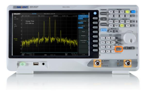
**NOTE:** The file type selected will also be mapped directly to the Save key located on the front panel. You can quickly open the file save dialog box by simply pressing Save once you have selected the file type.
