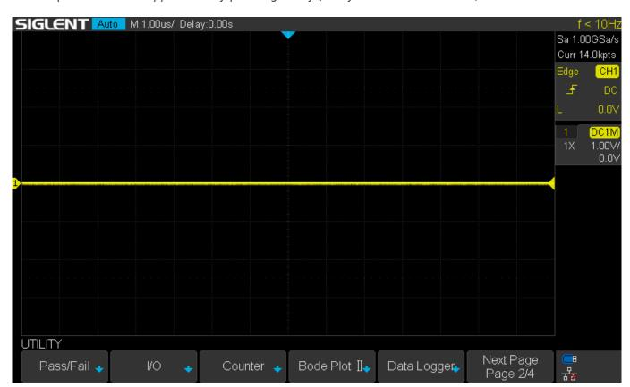
2. Configure the sweep parameters. For this example, we are going to simply change the end frequency to 200 kHz and the number of points to 200
