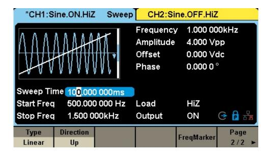
4. Set the marker frequency to 1.11 kHz and set the state to ON
