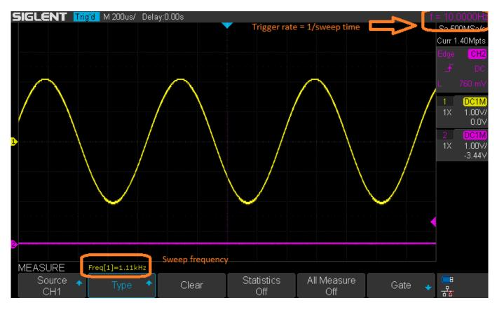
The frequency marker will output a pulse at the same time that the sweep frequency meets the setpoint for marker frequency.
