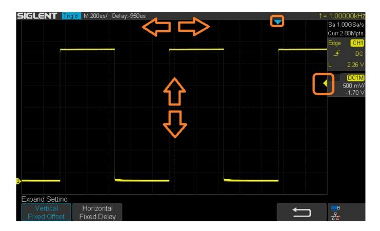
When we zoom around fixed positions, the horizontal offset and vertical positions are fixed on the display and the waveform is expanded around those points as shown here:
