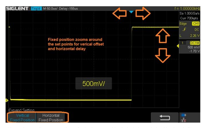
This new feature allows you to select a fixed reference position for both the vertical and hortizonal offset positions for the zoom. This makes for faster troubleshooting by minimizing the number of adjustments required to zoom on the area of interest.
