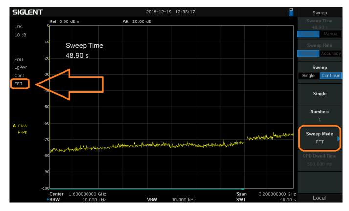
If the instrument dsplays a "sweep time error" or "RBW error", check the sweep mode, RBW, and span settings. You may need to select another sweep mode and perform the scan again.
