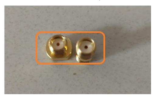
3.5 mm connectors have an air insulator:
