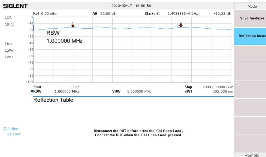
2) In the Reflection Measurement mode the user can modify certain spectrum analyzer parameters such as **Frequency, Amplitude, and BW**, in those related menus.
