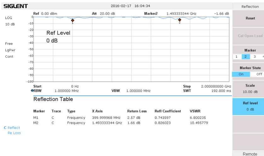
5) Press **Marker**, select a Marker (1-4), and Press **Marker status**->**On** to open multiple Markers. Move the position of the Marker and the Reflection Table will display the frequency, return loss, reflection coefficient and VSWR at that Marker point. The Scale is used to set the value of the grid's vertical scale. The Ref level sets the maximum value (top line) shown on the screen.
