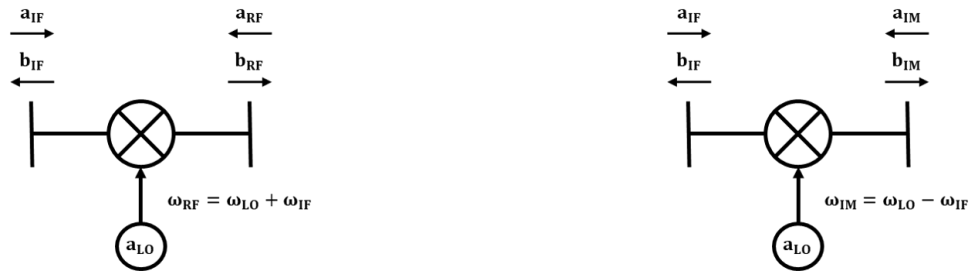
Schematic of a normal (a) and image (b) mixers showing incident and scattered waves
