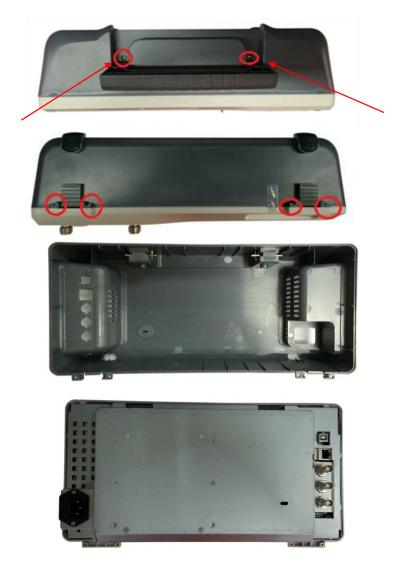
Figure 4-1 Removing the Rear Panel Screws
