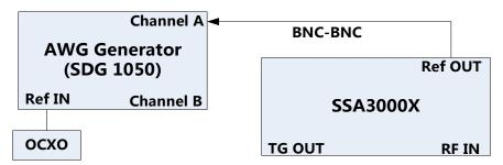
Figure 3-6 Connecting test instruments for frequency accuracy
