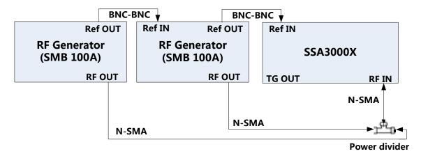
Figure 3-5 TOI verification connections
