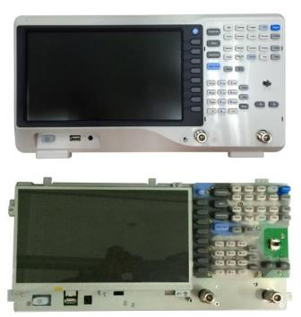
Figure 4-2 Removing the front panel
