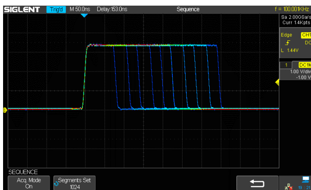
Segmented memory collection will store the waveform into multiple (up to 80,000) memory segments and each segment will store a triggered waveform, as well as the dead time information. The dead time between segments could be as small as 2 µs. All the segments can be played back using History function.
