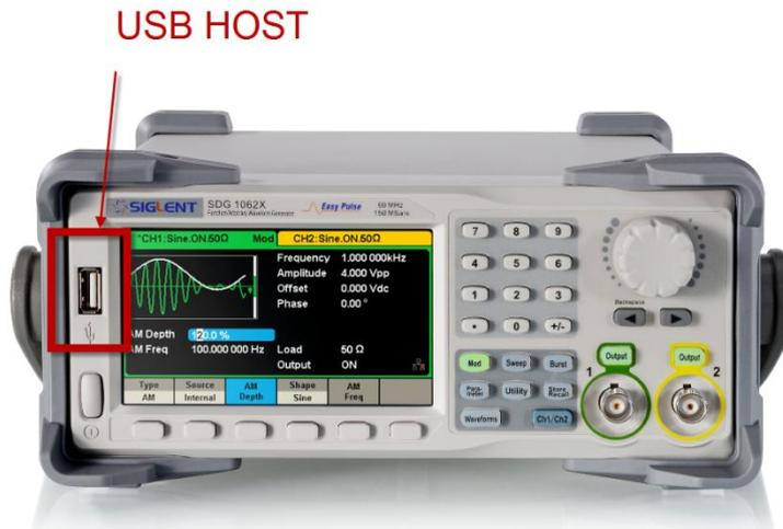
2. Press the **Utility** key on the front panel, and then softkey “System ->Page 1/2 -> Firmware Update”, to enter the interface of the file browser.
