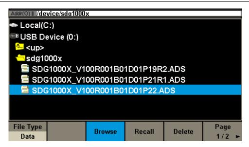
4. Press "Recall" to start the update. A progress bar is displayed during the update. After the update is completed, the generator will restart automatically.
