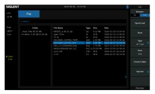
4. Press "Open/Load" to start the update. A progress bar is displayed during the update. When updating complete, the spectrum analyzer will restart automatically.
