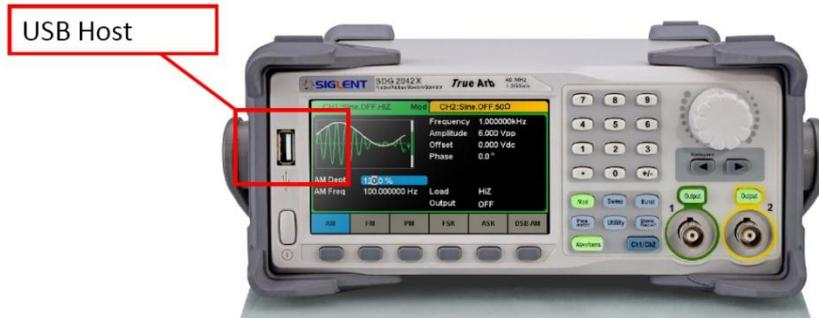
2. Press the **Utility** key on the front panel, and then softkey “System ->Page 1/2 -> Firmware Update”, to enter the interface of the file browser.
