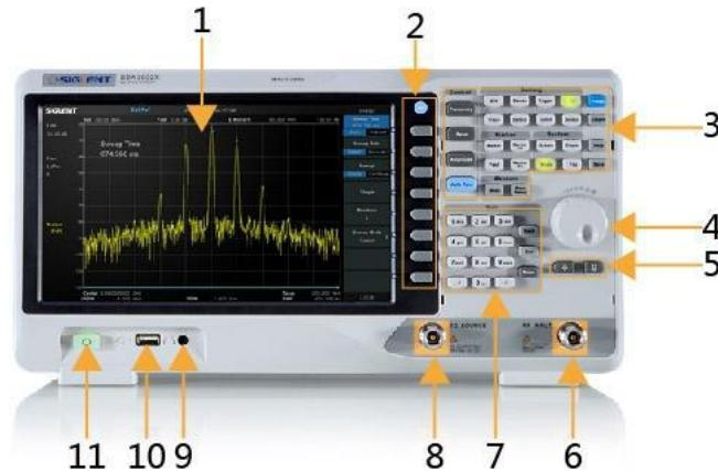
2. Press the **System** key on the front panel, and then softkey “System->System Info-> Firmware Update”, to enter the interface of the file browser.
